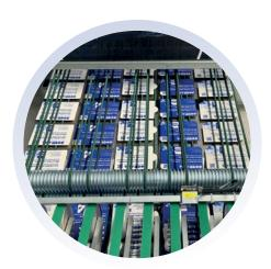
Optimized product transport thanks to round belts with spreading effect at the infeed.
