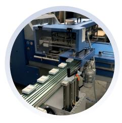
Transport the deck to downstream modules e.g. delivery belts, overwrappers, banding machines or similar.
