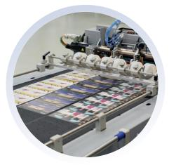
Vacuum belt for stable and careful transport in a shingled stream or as individual products.
