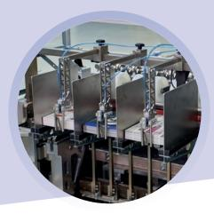
For a fast format change an optional set of bulkheads can be prepared outside the stack delivery.
